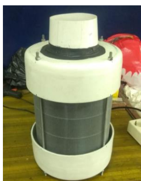
Gambar 5. High Efficiency Particulate Air (HEPA) filter dan Wadahnya
